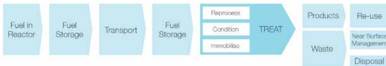
Figure 5 - Value chain for spent fuel management from reactor to final re-use, near surface management or disposal
