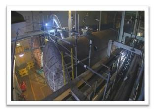
Trials continue for in-reactor tooling for PFR with tool 6 testing completed. In January, a fuel element carrier grab has been designed and manufactured to enable the removal of 37 carriers that are within PFR. This was the 4<sup>th</sup> reactor dismantling tool to be designed, delivered and successfully trialled during last financial year. The image shows the tool during final trials at the PFR cell 2 trial facility.
