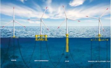
There are currently 4 main types of floating substructures that are being tested and developed.
